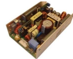
U Type (U-Chassis only): 3.2(W)x5(L)x1.5(H) inches.
